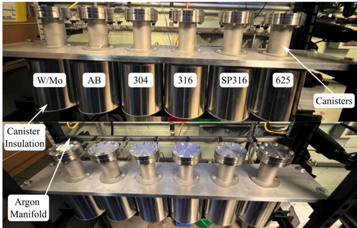
Fig. 1. Image showing the setup of the canisters holding the samples submerged in liquid lithium. The argon feed and canister insulation are also seen. Each canister is labelled with the corresponding material. Refer to Table 1 to compare the abbreviated names to full material names.
