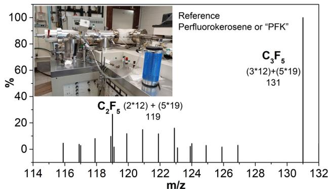
FIG. 3. Mass spectrometer coupled to U-trap (Dewar) and electron mass spectrum for stannane and perfluorokerosene (reference) compounds.
