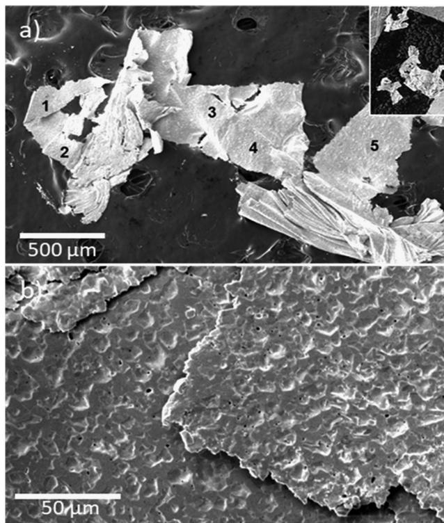
**FIG. 7.** SEM micrographs of Sn samples after conversion of  $\text{SnH}_4$  to Sn. (a) At  $500\ \mu\text{m}$  scale, points 1, 2, 3, 4, 5 denote the locations of semi-quantitative composition obtained by EDS of the Sn surface, and (b) at  $50\ \mu\text{m}$  scale, the picture is taken between points 1 and 2.
