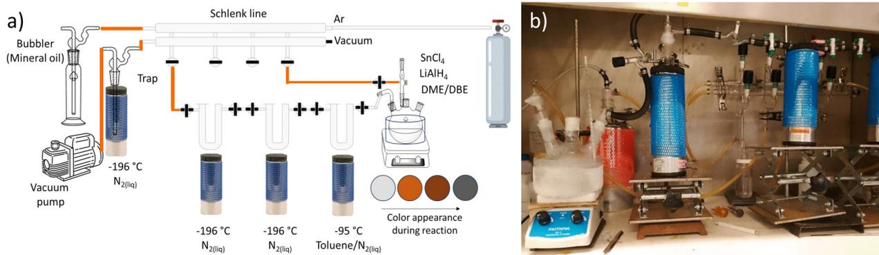
FIG. 1. (a) Schematic representation of the stannane synthesis using the Schlenk technique and (b) the real picture of the setup.
