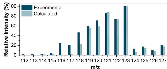
FIG. 4. Average positive EI mass spectrum of SnH<sub>x</sub><sup>+</sup> resulting from the ionization of SnH<sub>4</sub> obtained with an electron energy of 70 eV. The calculated spectra assume a  $68 \pm 3\%$ ,  $32 \pm 2\%$ ,  $0.7 \pm 0.02\%$  cracking pattern to SnH<sub>3</sub>, SnH<sub>2</sub>, and SnH, respectively, and the known isotopic abundances.
