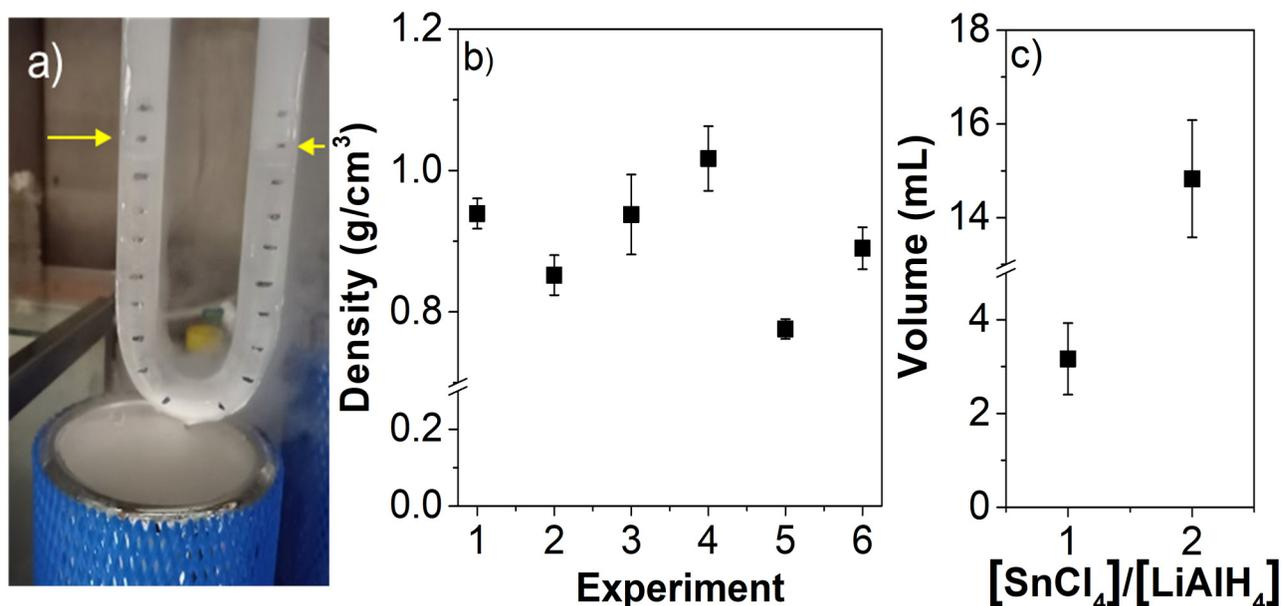
FIG. 2. (a) U-trap with SnH<sub>4</sub> liquid, (b) density values obtained at various experiments at  $-196\text{ }^{\circ}\text{C}$ , and (c) volume of SnH<sub>4</sub> according to the ratio of [SnCl<sub>4</sub>]:[LiAlH<sub>4</sub>].
