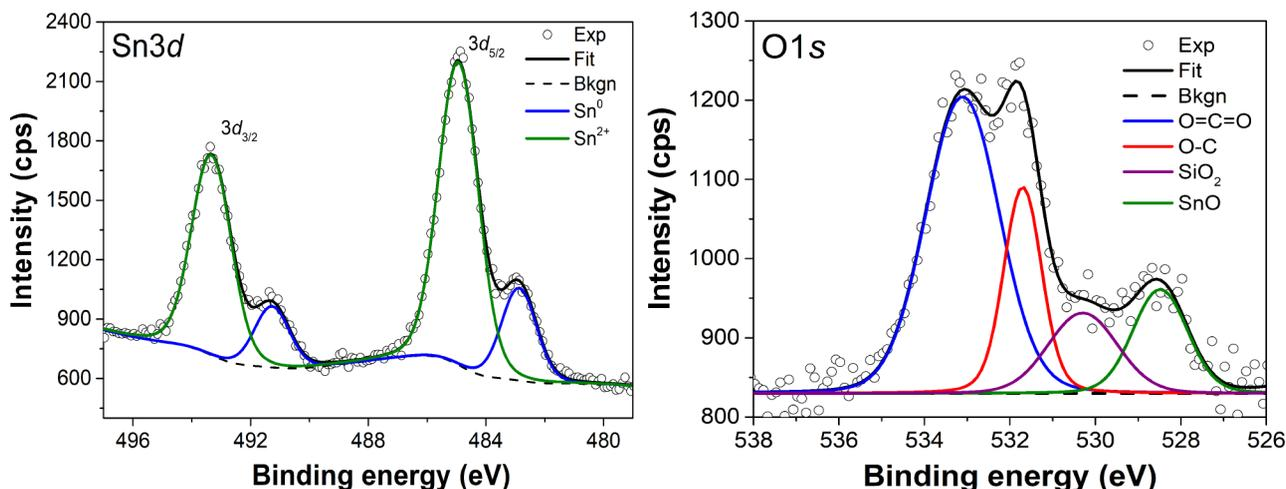
FIG. 6. XPS high-resolution spectra for Sn 3d and O 1s core energetic levels for Sn samples.
