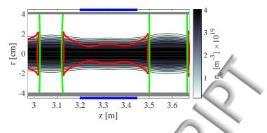
FIG. 5. Schematic of the ICH region in Proto-MPEX. The electron density profile in the ICH region is shown. The green contours represent the magnetic field value at which the ion cyclotron resonance at 7.5 MHz driving frequency exists. The red contours are locations of the Alfvén resonance at  $k_{\parallel} = 20 \text{ m}^{-1}$ . The ICH antenna is represented by the solid blue line and is separated from the plasma by an alumina tube which is represented by the grey line.
