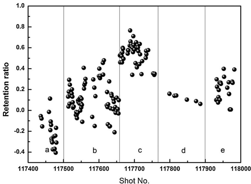
Fig. 8. Evolution of retention ratio as a function of discharge number, (a) FLiLi limiter without Li coating, (b) FLiLi limiter with Li coating, (c) Li coating (d) Mo limiter and (e) LIMIT limiter.
