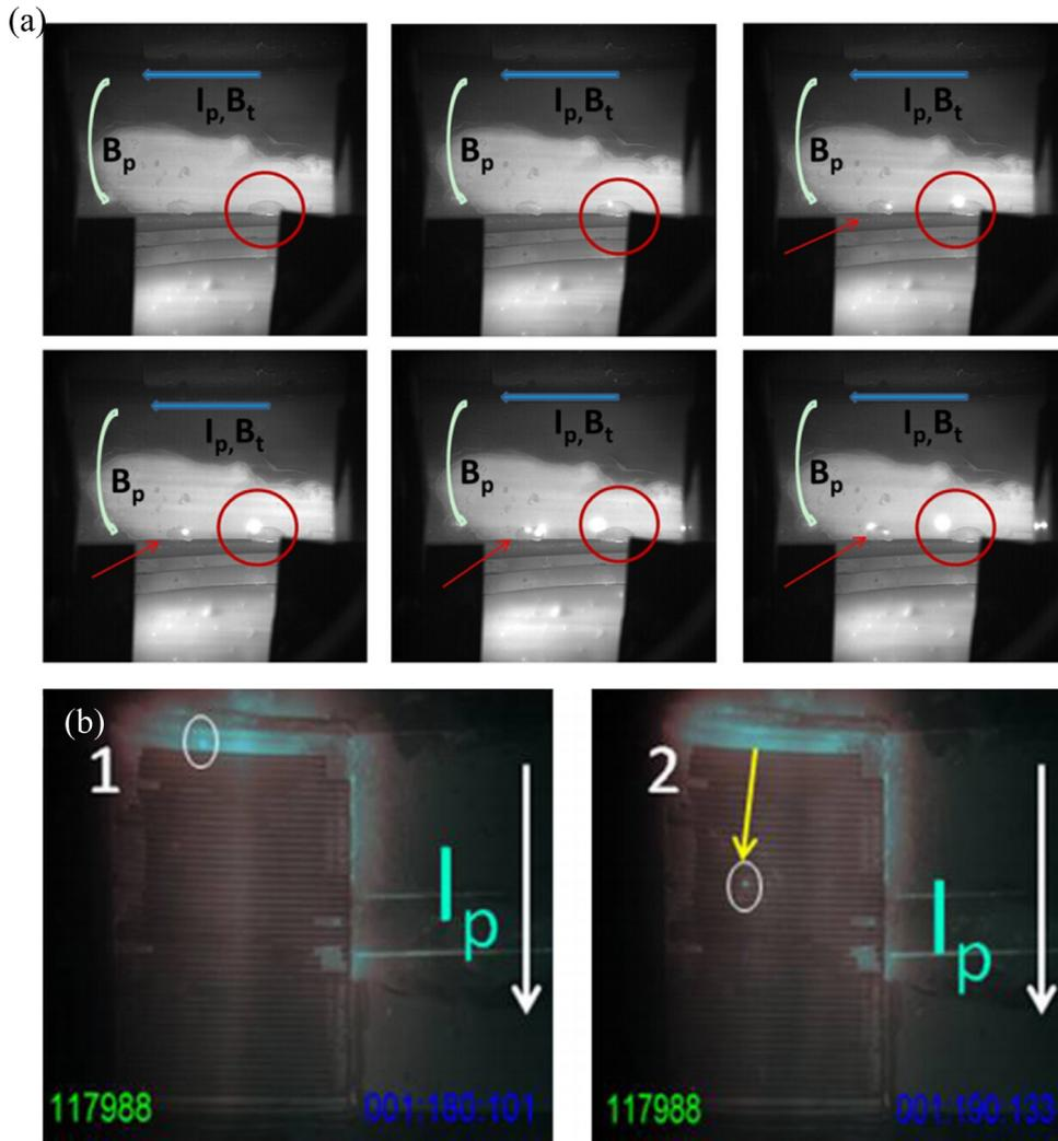
Fig. 2. Li droplet ejected from limiters by electromagnetic forces, (a) FLiLi limiter and (b) LIMIT limiter.
