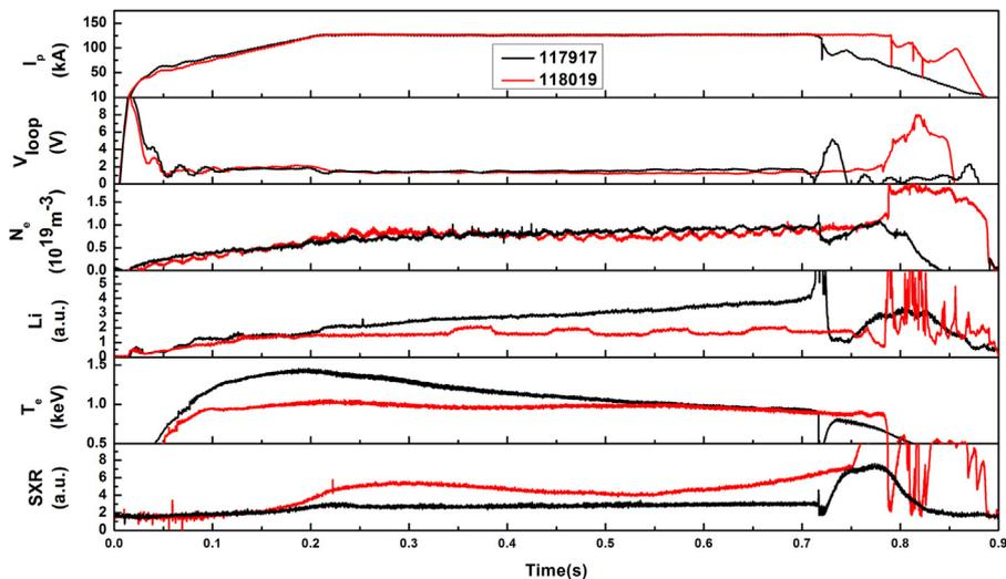
**Fig. 12.** Comparison of two discharges, #117917 shot employed LIMIT limiter discharge and # 118019 shot was the Mo limiter, plasma  $I_p$ , loop voltage  $V_{loop}$ , plasma density  $N_e$ , Li emission Li, core electronic temperature  $T_e$  and soft X-ray emission SXR.
