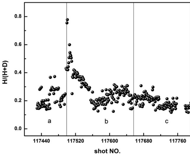
Fig. 7. Evolution of H/(H + D) ratio as a function of discharge number, (a) FLiLi limiter without Li coating, (b) FLiLi limiter with Li coating, (c) Li coating.
