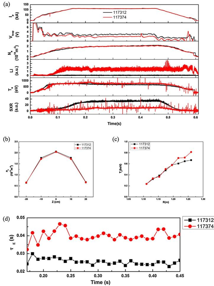
**Fig. 10.** Comparison of two discharges, #117312 shot was the Mo limiter discharge and # 117374 shot employed FLiLi limiter, (a) plasma current  $I_p$ , loop voltage  $V_{loop}$ , plasma density  $N_e$ , Li emission LI, core electronic temperature  $T_e$  and soft X-ray emission in core SXR, (b) profile of plasma density, (c) profile of electronic temperature and (d) energy confinement time.
