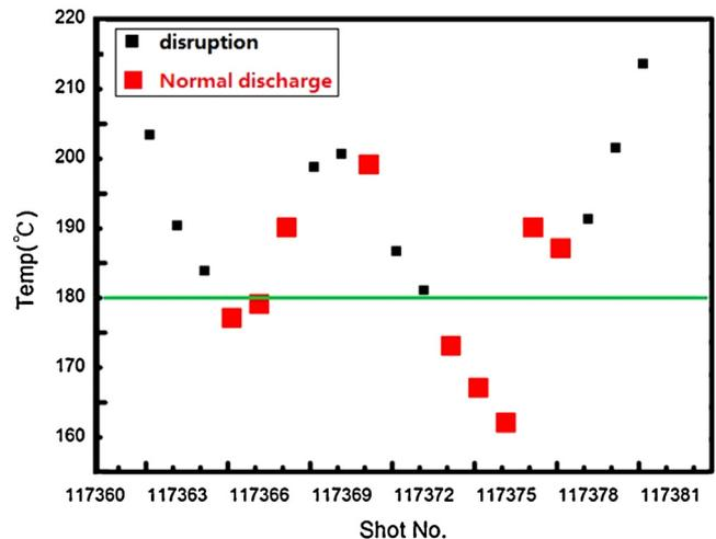
Fig. 3. The influence of temperature on the plasma discharge condition.
