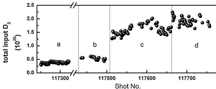
Fig. 6. Evolution of total input  $D_2$  as a function of discharge number, (a) Mo limiter, (b) FLiLi limiter without Li coating, (c) FLiLi limiter with Li coating, (d) Li coating.
