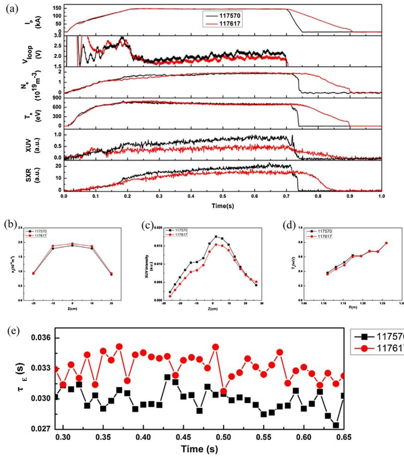
**Fig. 11.** Comparison of two discharges, #117570 shot was the Mo limiter discharge after Li coating and # 117617 shot employed limiter, (a) plasma  $I_p$ , loop voltage  $V_{loop}$ , plasma density  $N_e$ , core electronic temperature  $T_e$ , XUV emission and soft X-ray emission SXR in core, (b) profile of plasma density, (c) profile of XUV emission, (d) electronic temperature and (e) energy confinement time.
