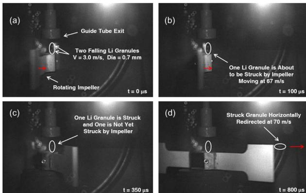
Fig. 2. Four sequence images of a granule injection event.
