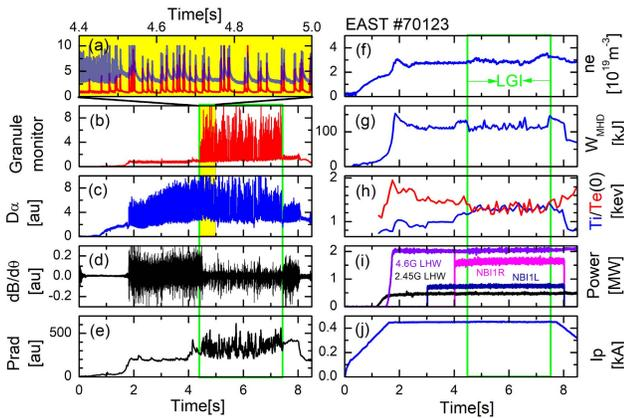
Fig. 7. Typical shot of ELM pacing by LGI during 4.4–7.4 s. (a) Granule monitor and ELM monitor by  $D\alpha$  signal. (b) Granule monitor by edge XUV signal. (c)  $D\alpha$  signal. (d) Magnetic perturbation. (e) Total radiation power from all XUV channels. (f) Line integrated plasma density. (g) Stored energy. (h) Core electron and ion temperature. (i) Heating scheme and injection power. (j) Plasma current.
