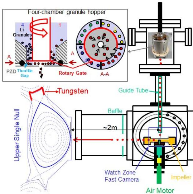
Fig. 1. Schematic of the injector hardware used in this paper. The spherical Li granules from one of four separate chambers fall through a narrow guide tube and are struck by the paddles of a rotating plastic impeller. The granules are thus horizontally redirected at higher speeds into the midplane of EAST upper single-null discharges.
