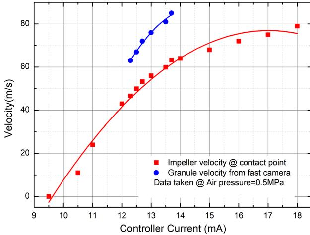
Fig. 4. Relationship among controller current, impeller velocity, and LGI velocity.
