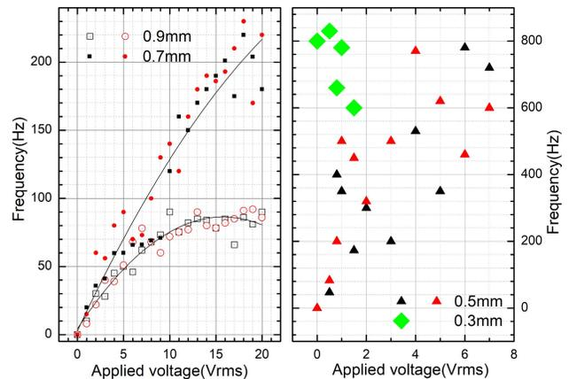
Fig. 3. Granule drop frequencies versus applied voltage to the PZD for four separate sized granules. Drop frequency versus voltage for the larger size granules (left). and Behavior of the smaller sized granules (right).
