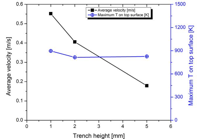
**Fig. 10.** Influence of the trench height on the average velocity and maximum surface temperature.
