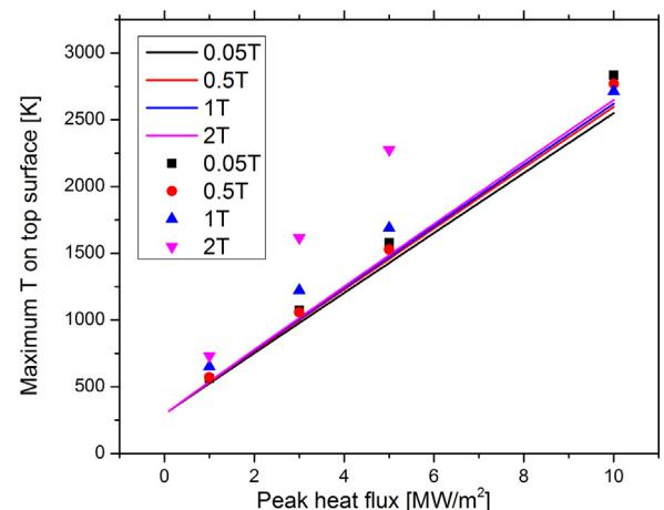
**Fig. 8.** Comparison of the maximum top surface temperature vs. peak heat flux, for magnetic fields in the range 0.05 T–2.0 T. The results from the 3D numerical model (points) are compared to the 1D model (solid lines) obtained in [7]. Simulations are run for heat transfer coefficient  $q' = 500 \text{ W}/(\text{m}^2 \text{ K})$ , and trench height = 5 mm.
