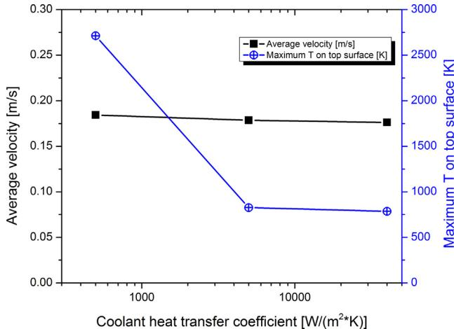
**Fig. 9.** Influence of the coolant heat transfer coefficient on the average velocity and maximum surface temperature.
