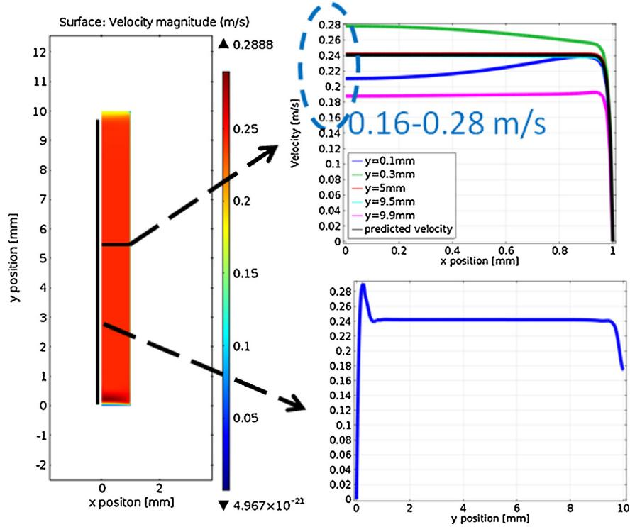
**Fig. 2.** Verification tests of the thermoelectric MHD flow on an infinite rectangular trench with an open surface. Left: magnitude of the flow velocity on a section of the trench. Top right: velocity profile along x direction at several y positions, and comparison with the theoretical result from [10]. Bottom right: flow velocity along the y direction.
