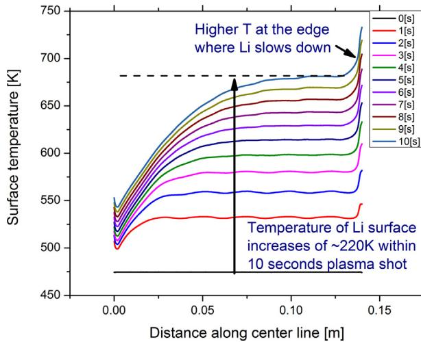
**Fig. 12.** Temperature increase of lithium during a 10-s plasma shot in HT-7, along a longitudinal line on the top surface at the center of trench.
