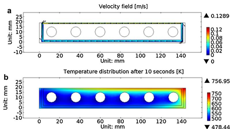
**Fig. 11.** (a) Velocity and (b) temperature of the cross section of the trenches after 10 s HT-7 plasma shot.
