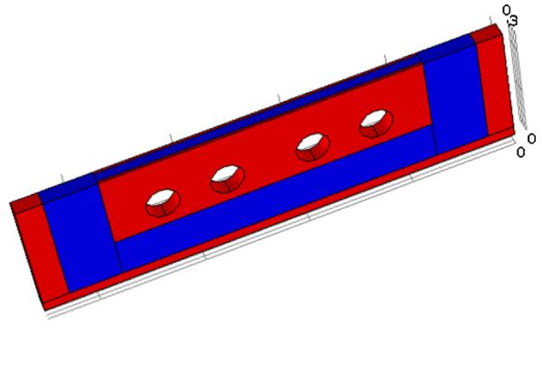
**Fig. 3.** Simulation domain, comprising the liquid lithium (blue) and the solid metal (red). The domain includes one trench, half of the metal walls, the four cooling channels, and the surrounding metal structure. (For interpretation of the references to color in this figure legend, the reader is referred to the web version of this article.)
