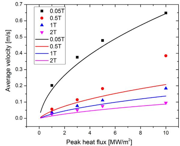
**Fig. 7.** Comparison of the average lithium velocity vs. peak heat flux, for magnetic fields in the range 0.05 T–2.0 T. The results from the 3D numerical model (points) are compared to the 1D model (solid lines) obtained in [7]. Simulations are run for heat transfer coefficient  $q' = 500 \text{ W}/(\text{m}^2 \text{ K})$ , and trench height = 5 mm.
