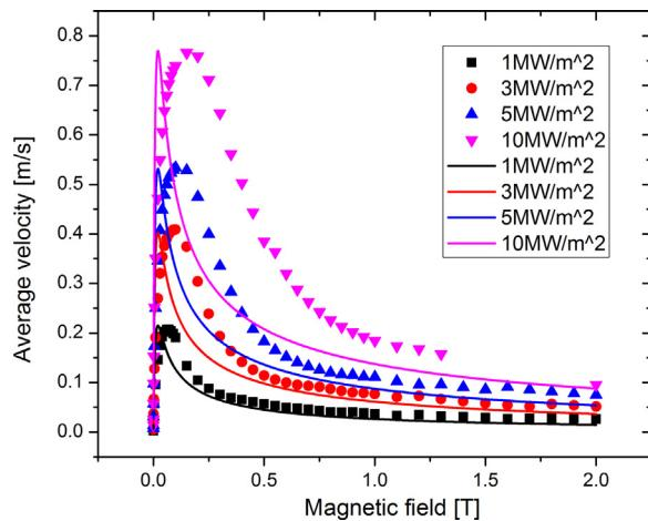
**Fig. 5.** Average lithium velocity vs. magnetic field, for different peak heat fluxes in the range 1.0–10 MW/m<sup>2</sup>. The results from the 3D numerical model (points) are compared to the 1D model (solid lines) obtained in [7]. Simulations are run for heat transfer coefficient  $q' = 500 \text{ W}/(\text{m}^2 \text{ K})$ , and trench height = 5 mm.
