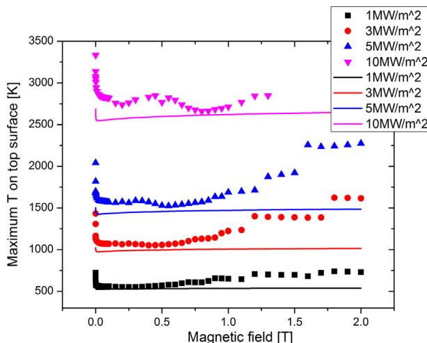
**Fig. 6.** Maximum top surface temperature vs. magnetic field, for different peak heat fluxes in the range 1.0–10 MW/m<sup>2</sup>. The results from the 3D numerical model (points) are compared with the 1D model (solid lines) obtained in [7]. Simulations are run for heat transfer coefficient  $q' = 500 \text{ W}/(\text{m}^2 \text{ K})$ , and trench height = 5 mm.
