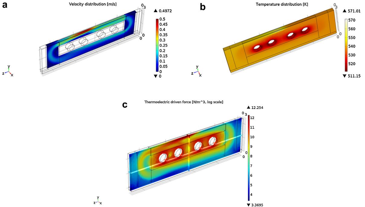
**Fig. 4.** (a) Flow velocity, (b) temperature, and (c) thermoelectric force (log scale), in LiMIT, as calculated from the 3D model.
