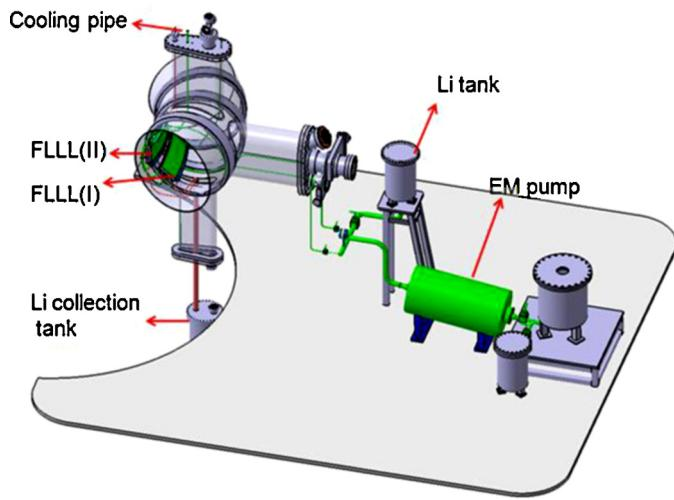
**Fig. 4.** Shown are the two thin-film FLLs tested in HT-7: FLL(I) developed at ASIPP and FLL(II) developed at PPPL. Also seen is the external support hardware needed to service the FLLs.
