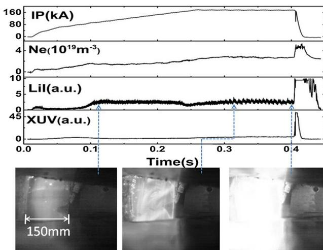
**Fig. 5.** Shown are images of the free-surface LLL located at the bottom of HT-7 (image rotated) showing Li effluxes at different phases of the discharge and the corresponding plasma parameters.
