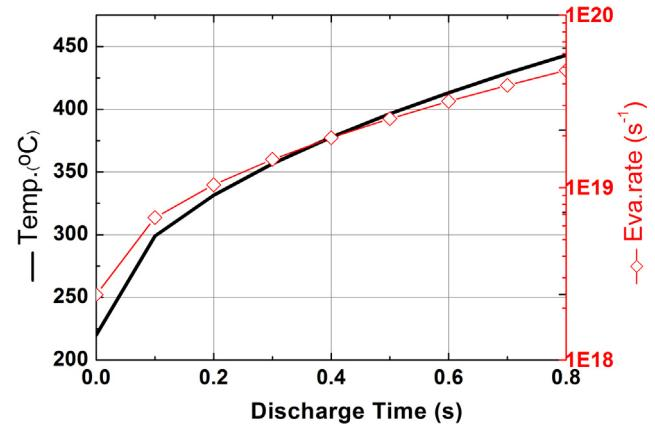
**Fig. 6.** Predicted Li surface temperature and evaporation rates during a typical OH discharge.
