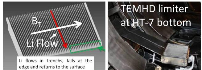
**Fig. 3.** The TEMHD liquid Li limiter showing the location and orientation of the Li liquid-filled trenches.
