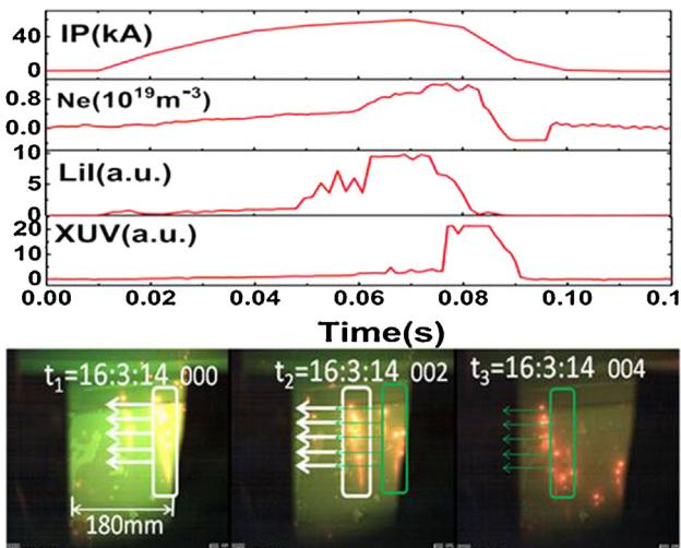
**Fig. 17.** Plasma performance and Li droplet movement with non-uniform Li flow. Over the 4 ms duration shown above, ejected droplets are captured moving at 20–100 m/s.
