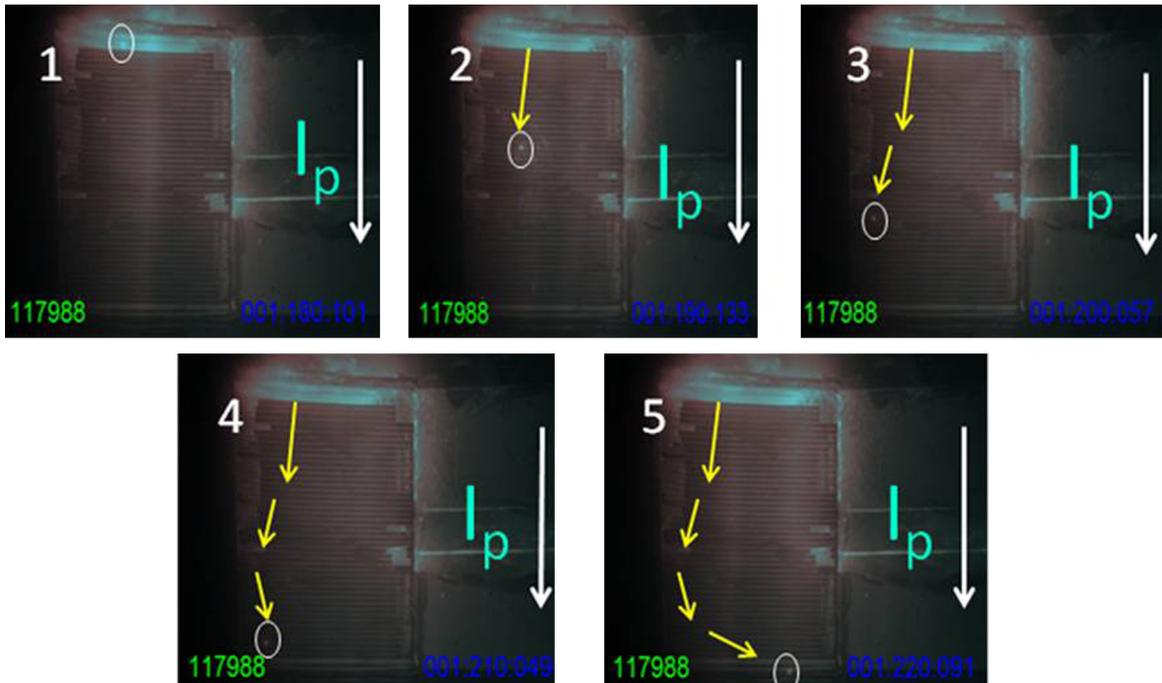
**Fig. 15.** The movement of a single liquid Li droplet captured fortuitously as it leaves the TEMHD FLLL and enters the plasma.
