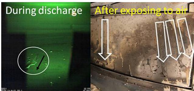
**Fig. 16.** Non-uniform Li flow along the SS plate of FLLL(I) was apparent during plasma operation and was consistent with the Li remnants found after exposure to air (images rotated).
