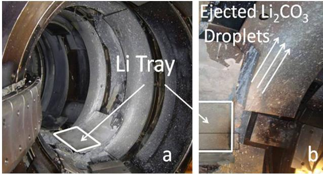
**Fig. 10.** Deposited spots of Li/Li<sub>2</sub>CO<sub>3</sub> on the walls of the vacuum vessel seen near the LLL after exposure to air.
