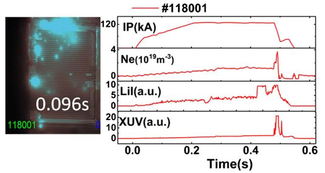
**Fig. 14.** Liquid Li ejection from the TEMHD FLLL and a subsequent plasma disruption.
