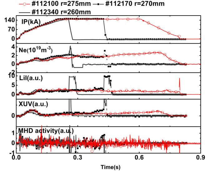
**Fig. 11.** Comparison of three plasmas run on a free-surface LLL as the radial position of the limiter was changed.
