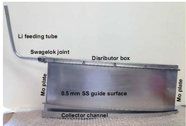
**Fig. 18.** Shown is the plasma facing surface of FLLL(II). During plasma operation, a thin wetted film of liquid Li flowed through holes spaced 0.8 mm apart in the manifold at the top to a collector channel at the bottom and eventually to an external Li storage tank (see Fig. 4).
