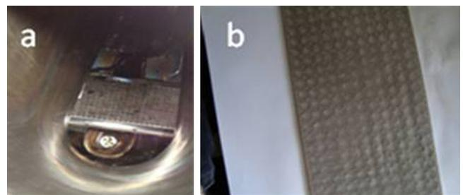
**Fig. 2.** Photos of LLL with (a) the original CPS configuration with wires and (b) a solid SS plate with many holes.
