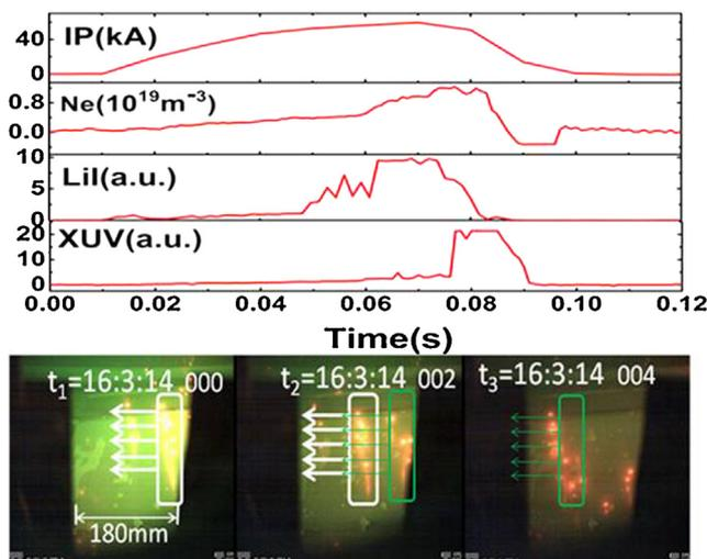
**Fig. 17.** Plasma performance and Li droplet movement with non-uniform Li flow. Over the 4 ms duration shown above, ejected droplets are captured moving at 20–100 m/s.
