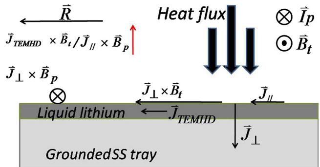
**Fig. 8.** Basic forces acting on free standing liquid Li.
