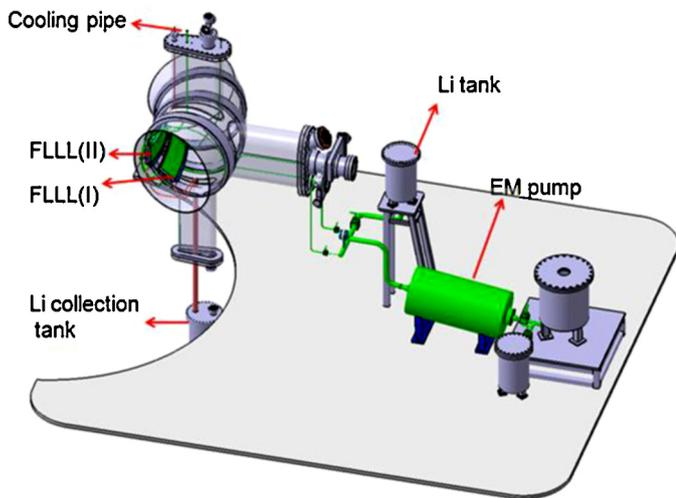
**Fig. 4.** Shown are the two thin-film FLLs tested in HT-7: FLLL(I) developed at ASIPP and FLLL(II) developed at PPPL. Also seen is the external support hardware needed to service the FLLs.
