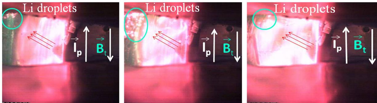
Fig. 9. Liquid Li movement in and droplet ejection from the LLL located at the bottom of HT-7 (image rotated).
