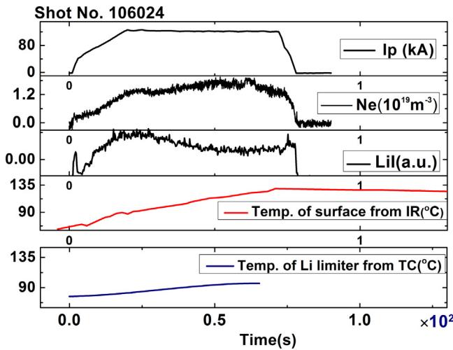
**Fig. 7.** Basic discharge parameters of a typical OH discharge run against a solid Li limiter with embedded thermocouples and monitored with an IR camera.
