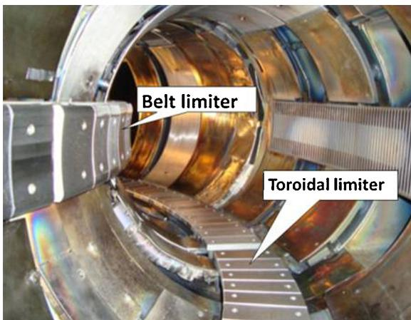
**Fig. 1.** Inner structures of HT-7.
