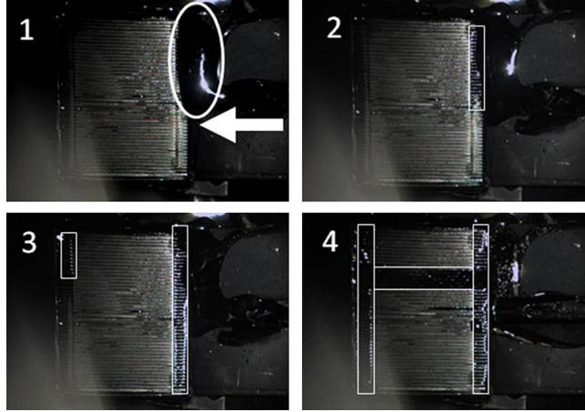
**Fig. 13.** Time-lapse photographs of liquid Li injection into the TEMHD FLLL. The boxes drawn on the figures show which parts of the structure have Li all the way to the surface. Even in frame 4, most of the surface does not have lithium present.
