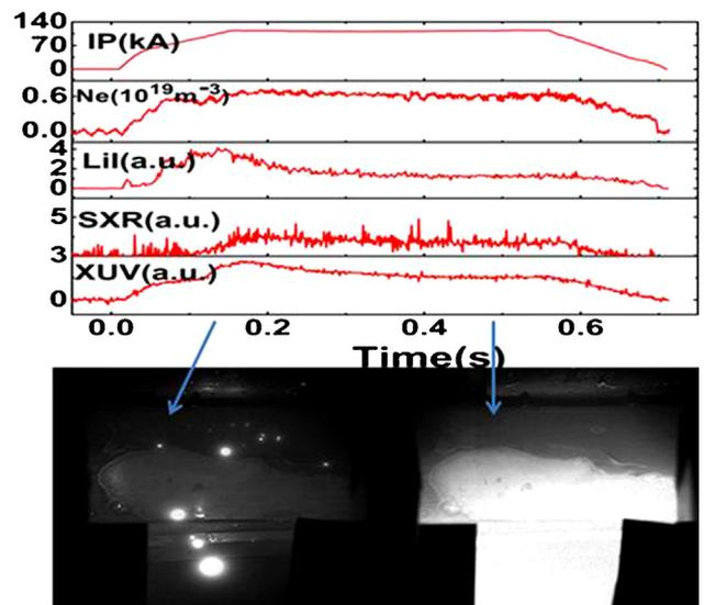
**Fig. 19.** Liquid Li behavior and plasma performance with thin and uniform Li flow exhibited with FLLL(II).
