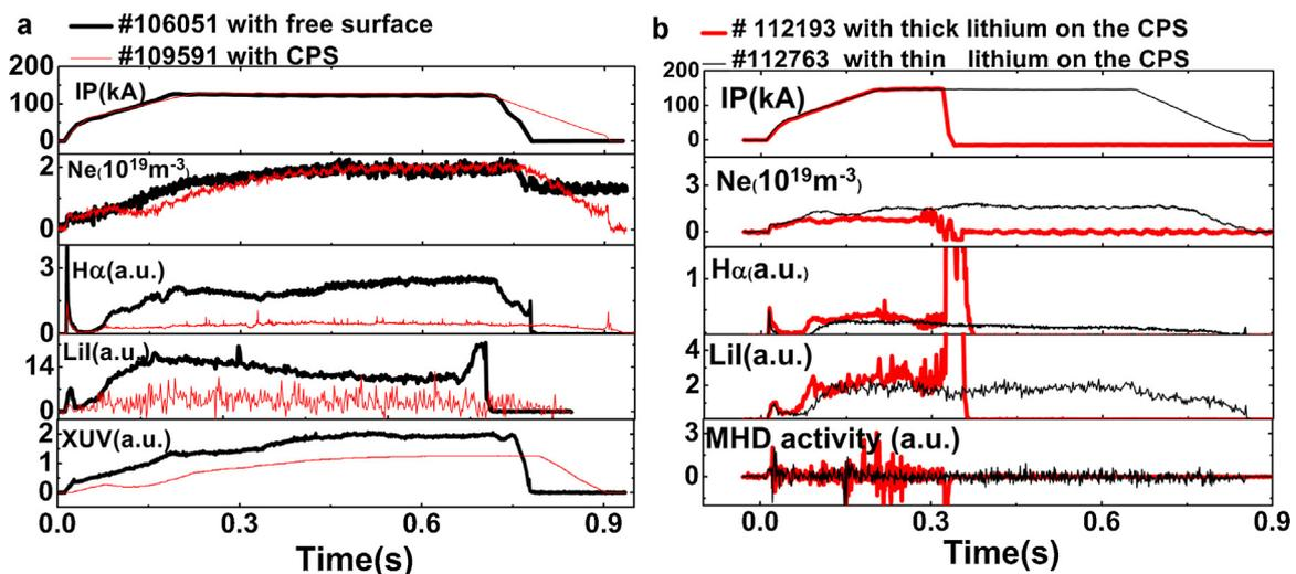
Fig. 12. Comparison of plasma discharges with different situations, (a) between free surface and CPS, (b) between thick and thin Li on the CPS.
