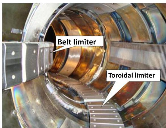
Fig. 1. Inner structures of HT-7.
