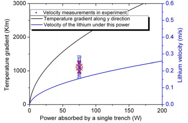
**Figure 6.** Plot of equations (3) and (5) versus the power absorbed by a trench. Experimental measurements of velocity from the particle tracking method and their mean (red circle) are also shown.
