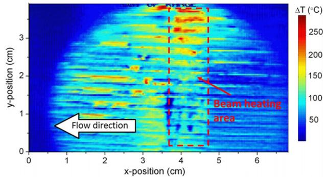
**Figure 4.** IR temperature measurement of the temperature increase during 20 s heating period. The initial temperature distribution has been subtracted and the lithium emissivity is assumed to be 0.05. Some of the hot and apparently cold spots are due to saturation of the camera from stationary impurities.
