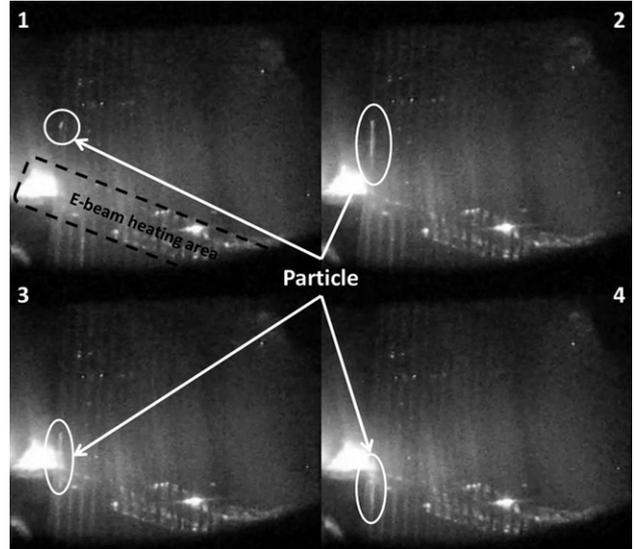
**Figure 3.** Flow measurements of the lithium using a Canon SX200IS movie camera with a frame rate of 25 frames per second. The heat stripe is perpendicular to the trenches as shown in the first frame. These four frames show a particle flowing along one of the trenches. The elongation of the track is due to the movement during the exposure of each frame.
