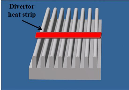
**Figure 1.** The LiMIT concept: metal tiles with radial trenches containing lithium. The trenches run in the radial (poloidal) direction such that they lie primarily perpendicular to the toroidal magnetic field and the divertor heat stripe.
