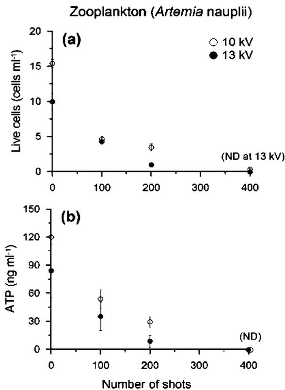
**Fig. 2** Effects of applied voltages and pulse numbers on viability of zooplankton (*Artemia nauplii*) determined by **a** live and dead cell counts and **b** ATP content measurements. When bars are not shown, 1 SD is less than size of the symbol ( $n=3$ ). ND; not detected
