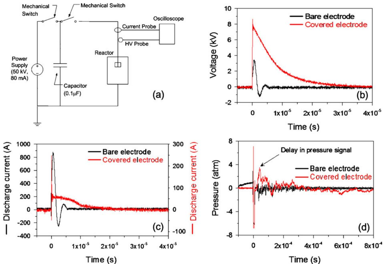
**Fig. 1** Description of pulsed high-voltage system. **a** Schematic diagram of the system and a treatment reactor. **b** Voltage and **c** current waveform of two different discharges at 7.1 kV. Note
