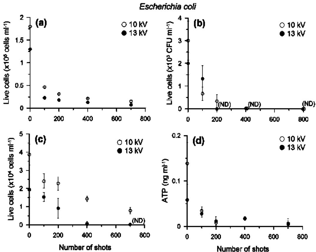
**Fig. 4** Effects of applied voltages and pulse numbers on viability of *Escherichia coli* determined by **a** live and dead cells counts, **b** membrane filter method (mEndo), **c** enzyme
