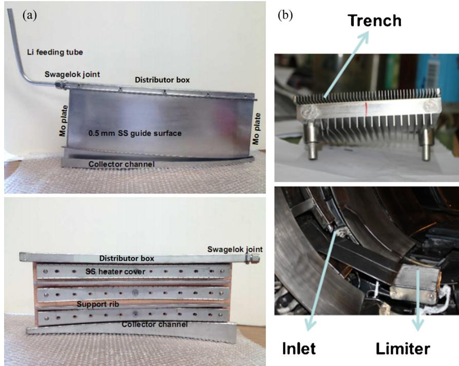
**Fig. 1.** Structures of the FLiLi limiter (a) and LIMIT limiter (b).
