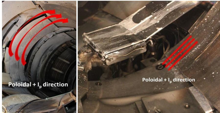
**Fig. 5.** The picture of flowing liquid lithium limiter and trace of lithium emission after experiment.
