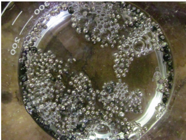
FIG. 4. Lithium pellets post production floating in Multi-Therm PG-1 mineral oil.
