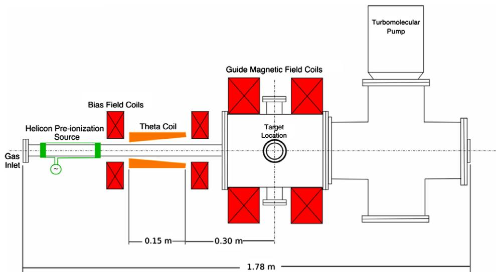
Fig. 1. Schematic drawing of the top view of the ELM simulating plasma gun (ESP-gun) at the University of Illinois, Urbana-Champaign.
