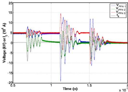
Fig. 2. Voltage and current waveforms for three consecutive pulses for a total pulse length of 1 ms.
