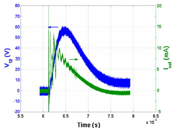
Fig. 3. Triple Langmuir probe waveforms ( $V_{12}$  and  $i_{\text{sat}}$ ) acquired during a 450 J discharge.  $V_{12}$  is proportional to  $T_e$ , and  $i_{\text{sat}}$  is proportional to  $n_e$ .
