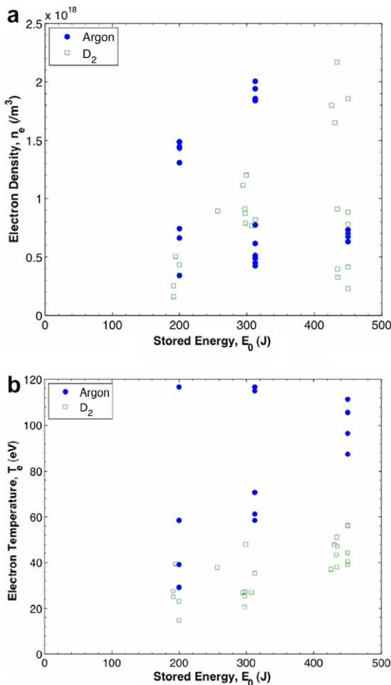
Fig. 4. Peak electron density measurements (a) and temperature (b) as a function of discharge energy.
