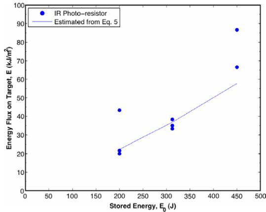
Fig. 5. Energy flux measured from the IR photo-resistor measurements (●) and estimated from the triple Langmuir probe (TLP) measurements (—).
